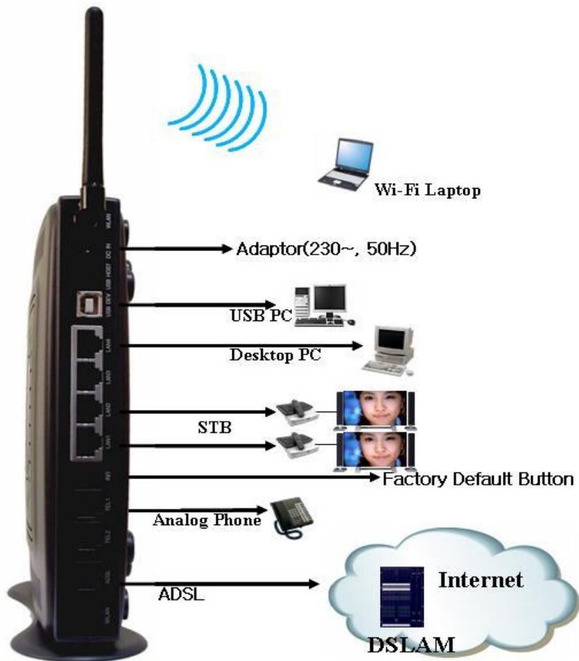
<Figure 2> DV-2010 Cable connection
